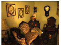
**Figure 4**. Global motion estimation followed by temporal sigma filtering. Because of the low SNR of the signals, the sigma filter was unable to differentiate noise from different image content caused by motion.
