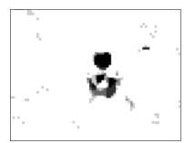
**Figure 6.** Map representing contributions to the temporal sigma filter. Most of the background regions used data from all six images (white regions) while some blocks near the person's hands and head used only the reference image and, therefore, achieved no noise reduction at all.
