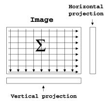
*Figure 1.* Integral projections. The two-dimensional image is converted into two one-dimensional projection vectors by summing along rows, and down columns.
